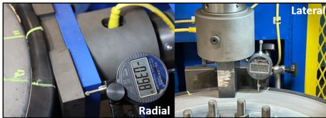
Figure 8: Dial Indicator Locations (for deflection measurement)
