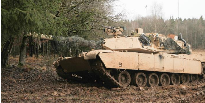
Figure 14: M1 Abrams with mud lodged inside roadwheels
